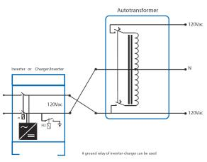
Split phase: 120VAC to 120/240VAC (Internal ground relay of inverter/charger may be used)
