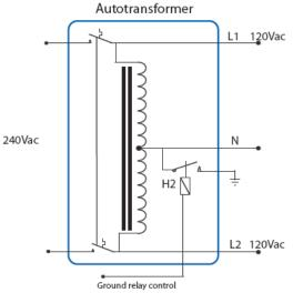
Autotransformer: schematic diagram
