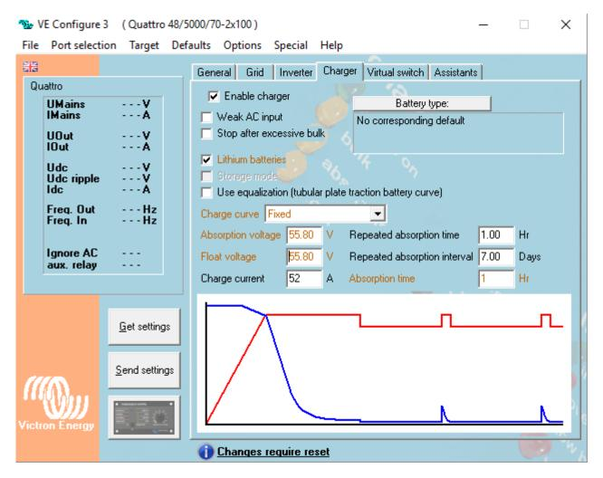
■ When setting up the ESS Assistant select LiFePO4 battery and enter the Ah value for the LiTE (or the combination of LiTE for a parallel battery system) as per the Ah rating provided in the LiTE specification sheet eg. LiTE 5/4 = 100Ah.
