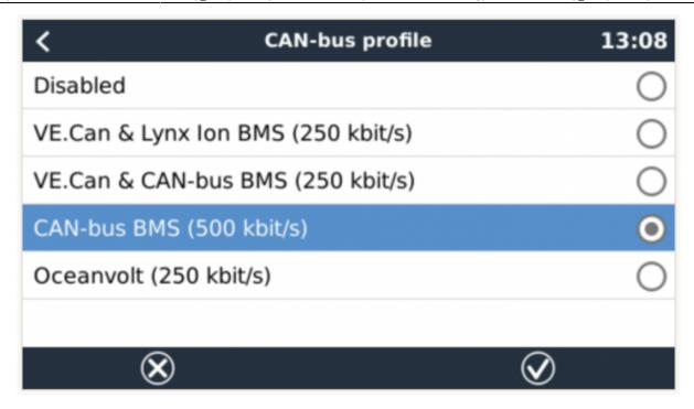
**▼** Confirm that the Freedom Won LiTE is showing in the device list (top of the menu structure) as per below
