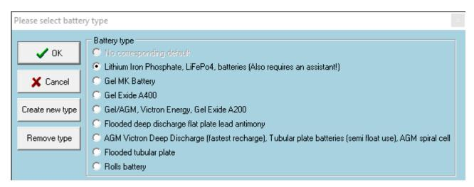
► Set Charger Settings. The charge voltage values are overridden by the LiTE but should be set correctly regardless for redundancy. The charge current should be set according to the user's requirements **but** this value combined with all other charge sources cannot exceed the charge limit of the battery – it is possible to select "Limit Charge Current" on the GX-device as an additional measure to prevent the total system charge current from exceeding the charge capacity of the LiTE.
