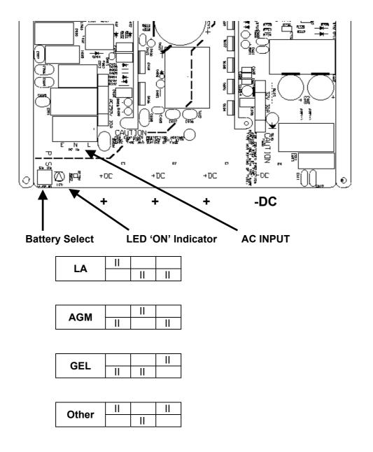
FIGURE 1 INPUT/ OUTPUT CONNECTIONS
